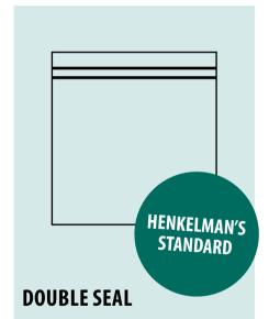
Double seal is Henkelman's standard. It consists of two 3.5 mm convex seal wires, especially suitable for basic sealing needs. For every application in every branche, from hospitality to the vacuum packaging of both food and non-food.
