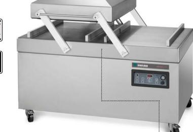
PUMP CAPACITY 100 m³/h MACHINE CYCLE 15-40 sec CHAMBER DIMENSIONS 760 x 660 x 280 mm MACHINE DIMENSIONS 1210 x 1545 x 1105 mm SEAL BARS 2 x 660 mm WEIGHT 462 kg VOLTAGE 400V-3-50Hz POWER 2,2-4,8 kW
